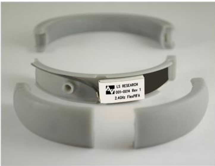
Figure 40: FlexPIFA integrated into bracelet
