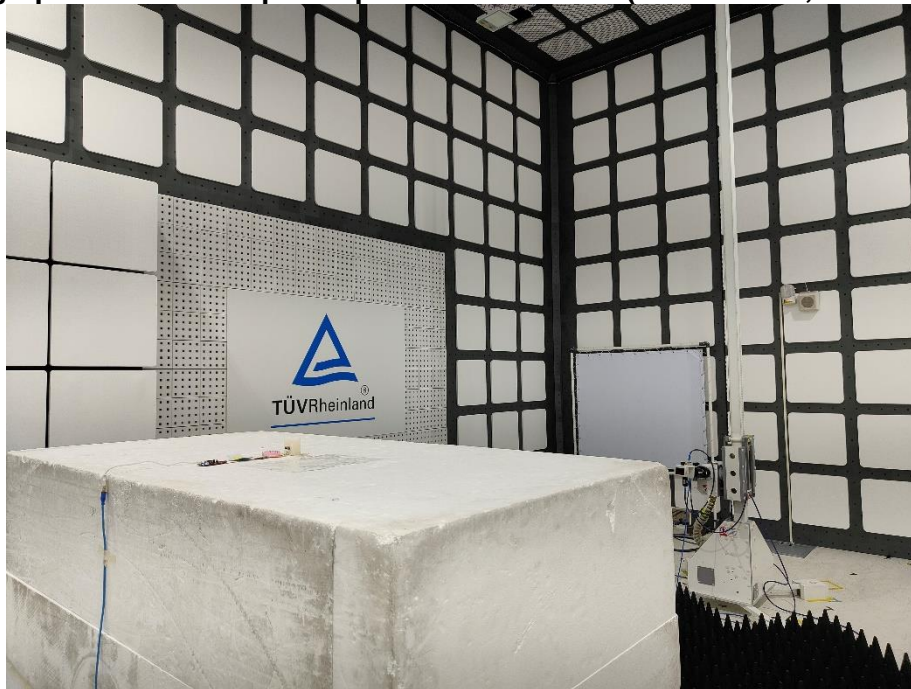
Photograph 40: Test Setup for Spurious Emissions (Back View 4, 2 nd Source)
