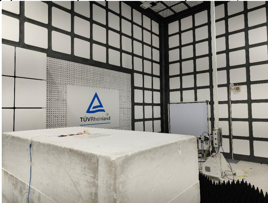
Photograph 20: Test Setup for Spurious Emissions (Back View 4, Main Source)
