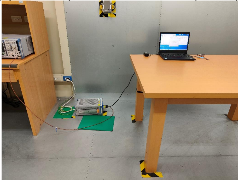
Photograph 14: Test Setup for Mains Conducted Emissions (Back View)
