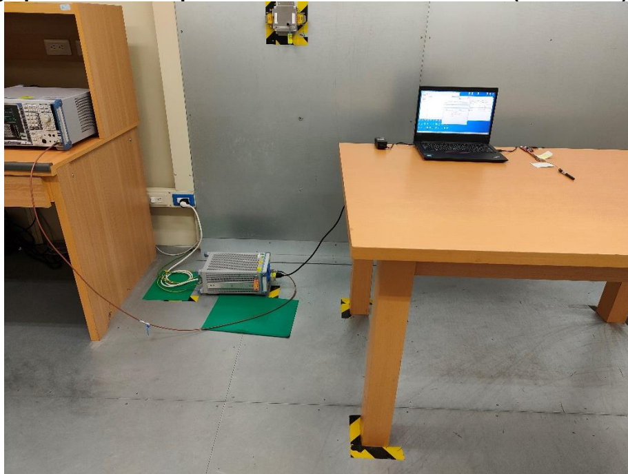
Photograph 41: Test Setup for Mains Conducted Emissions (Front View)
