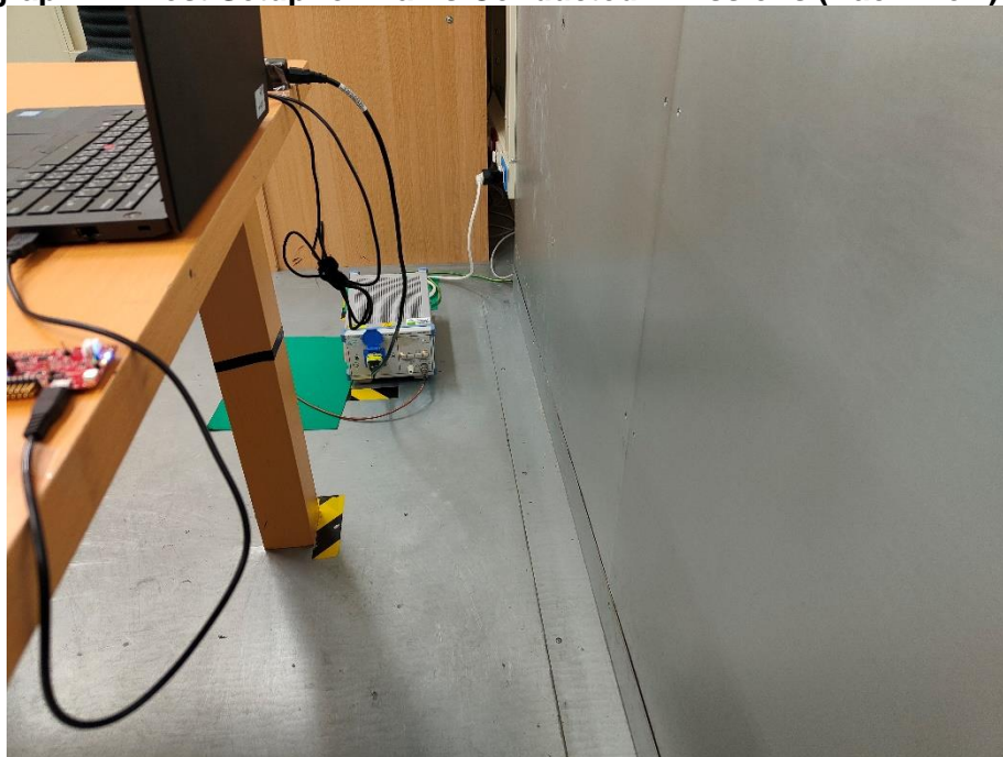
Photograph 14: Test Setup for Mains Conducted Emissions (Back View)
