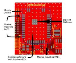
The top layer (underneath the module) of the host PCB must be ground with as many GND vias as possible.
