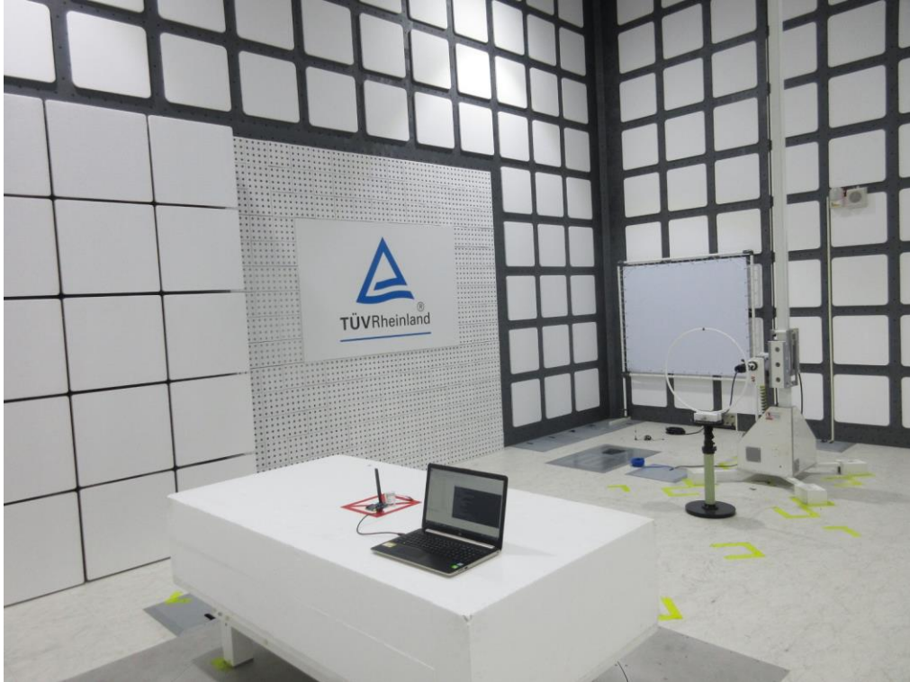
Photograph 5: Set-up for Spurious Emissions (Back View 3)
