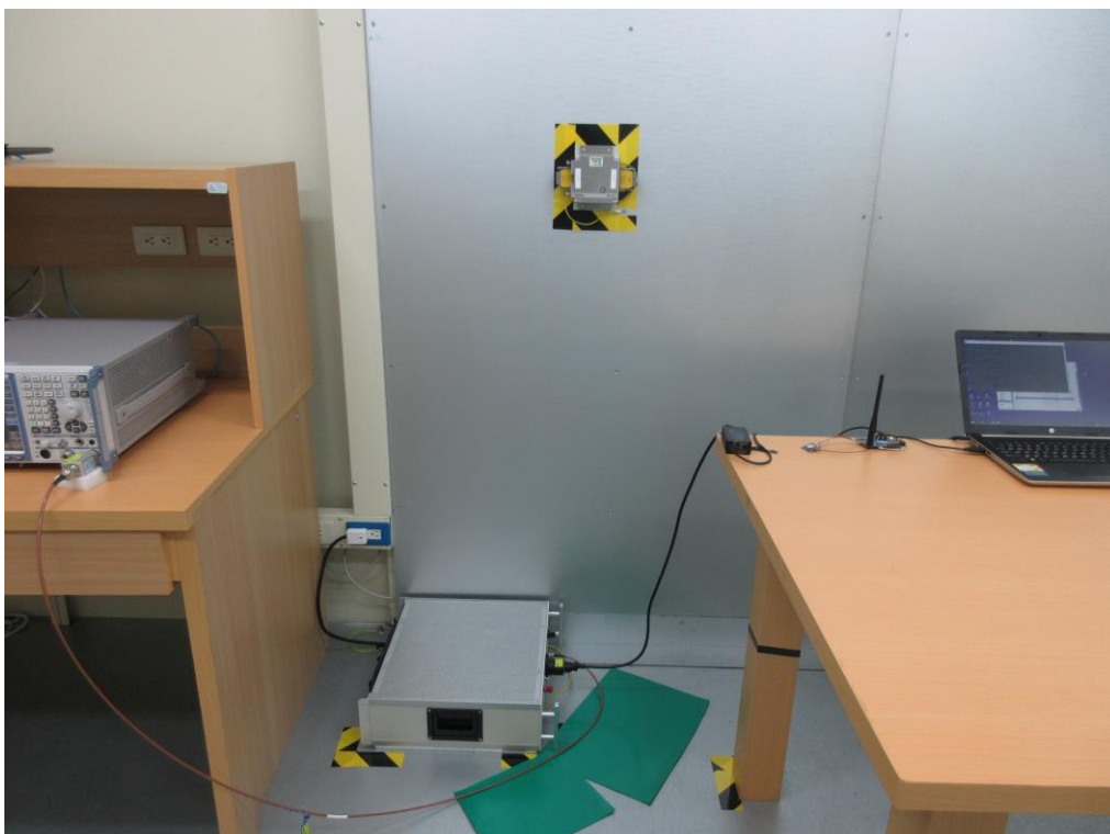
Photograph 6: Set-up for Mains Conducted testing (Front View)
