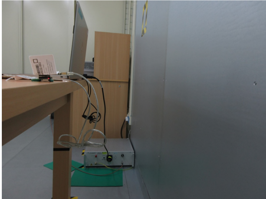
Photograph 7: Set-up for AC Mains Emissions (Back View)
