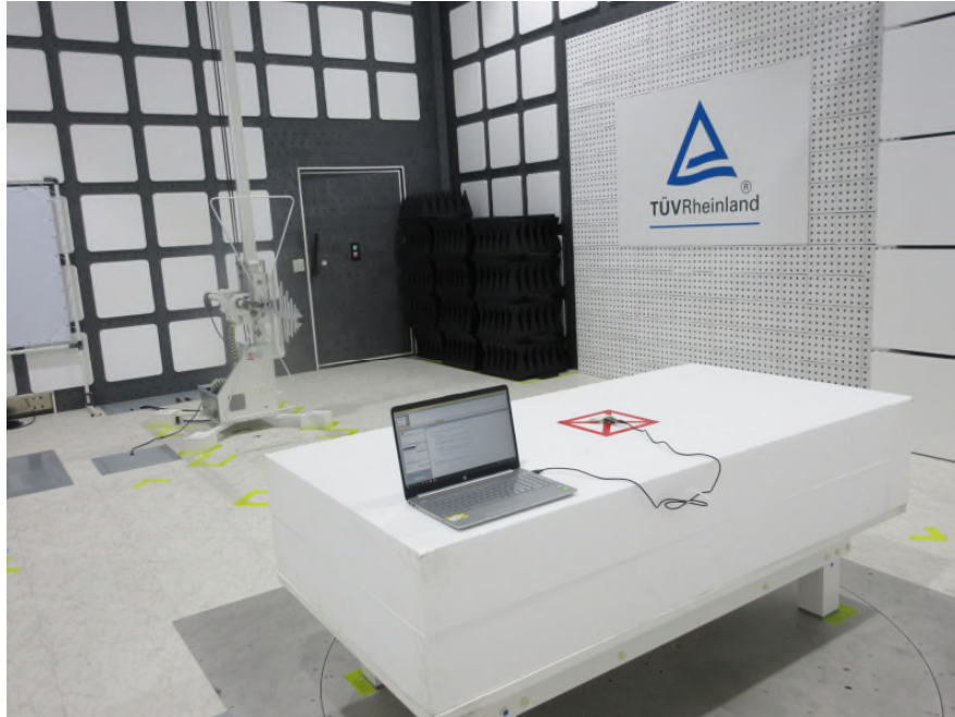
Photograph 3: Set-up for Spurious Emissions (Back View 1)
