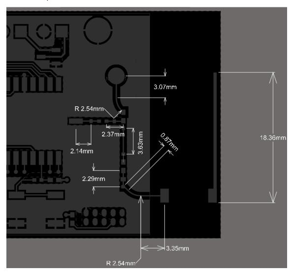
Below board shows the bottom layer layout of the reference board directly beneath the RF traces
