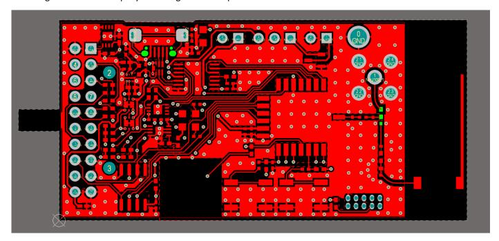
Below figure shows the Top layer layout of the reference host board focussed on RF traces. The snapshot also indicates the critical dimensions that are required to be replicated in the design to maintain compliance.
