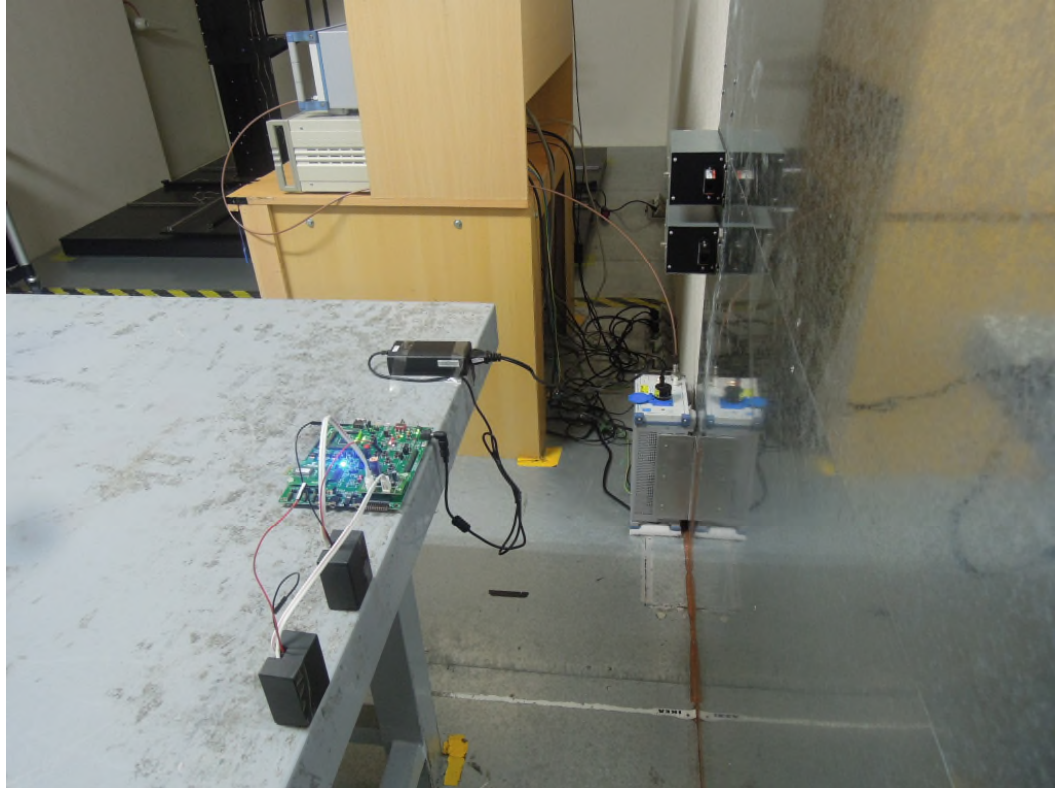
Set-up for Mains Conducted testing (Front View)
