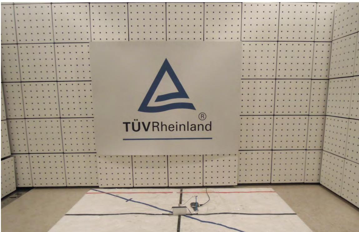
Photograph 7: Set-up for Spurious Emissions (Front view 1) - RFMTA331215IMAB701-ANT
