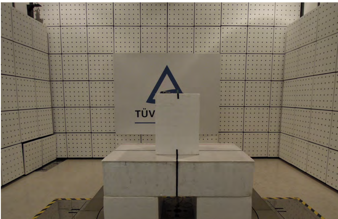
Photograph 27: Set-up for Spurious Emissions (Front View)- W3525B039-ANT
