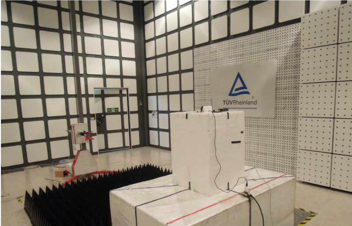
Photograph 17: Set-up for Spurious Emissions (Back View 3) - RFPCA381013IMAB701-ANT
