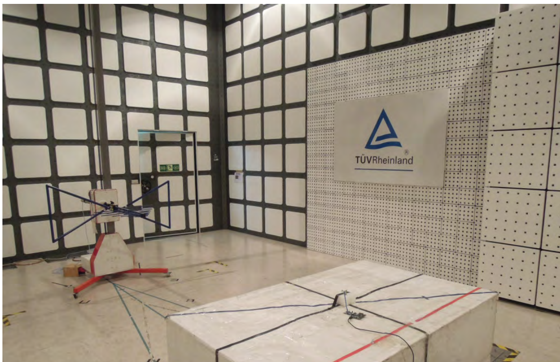
Photograph 15: Set-up for Spurious Emissions (Back View 1) - RFPCA381013IMAB701-ANT
