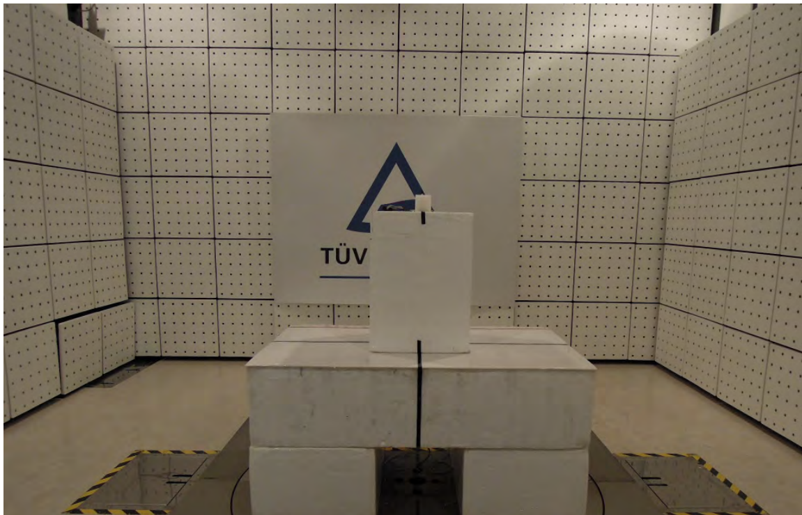
Photograph 25: Set-up for Spurious Emissions (Front View)- ACC-RN-SMA-S-DS -ANT
