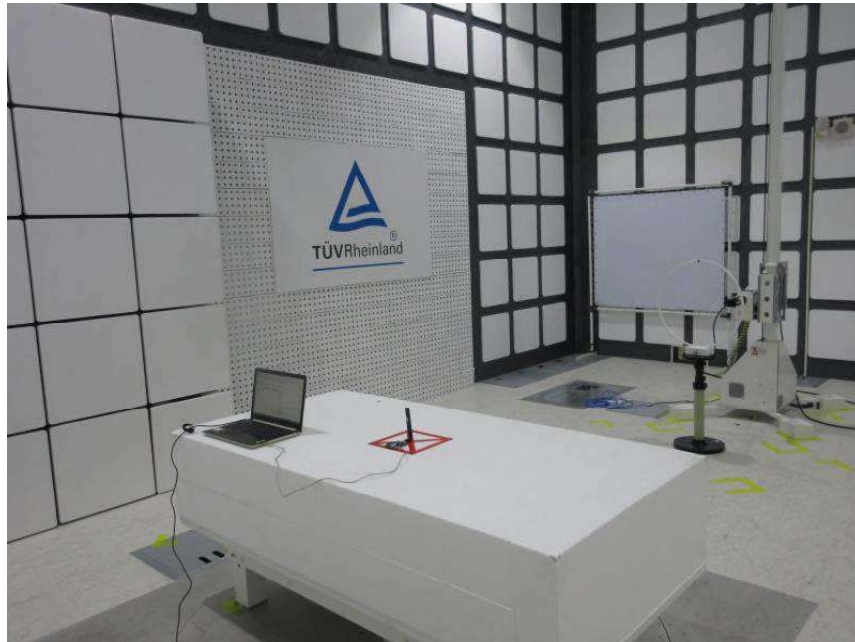
Photograph 5: Set-up for Spurious Emissions (Back View 3)
