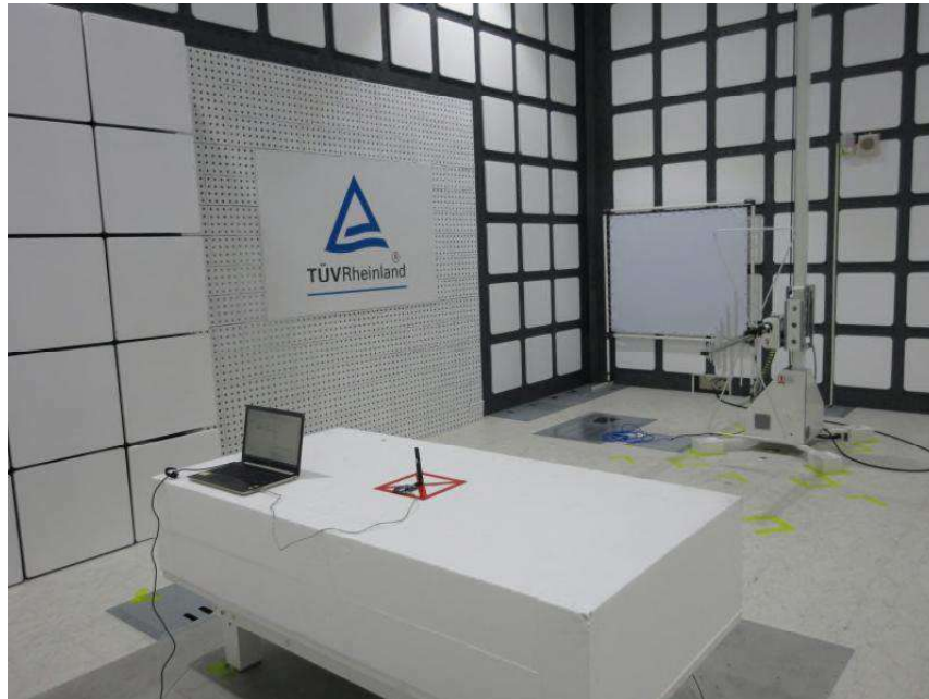
Photograph 3: Set-up for Spurious Emissions (Back View 1)
