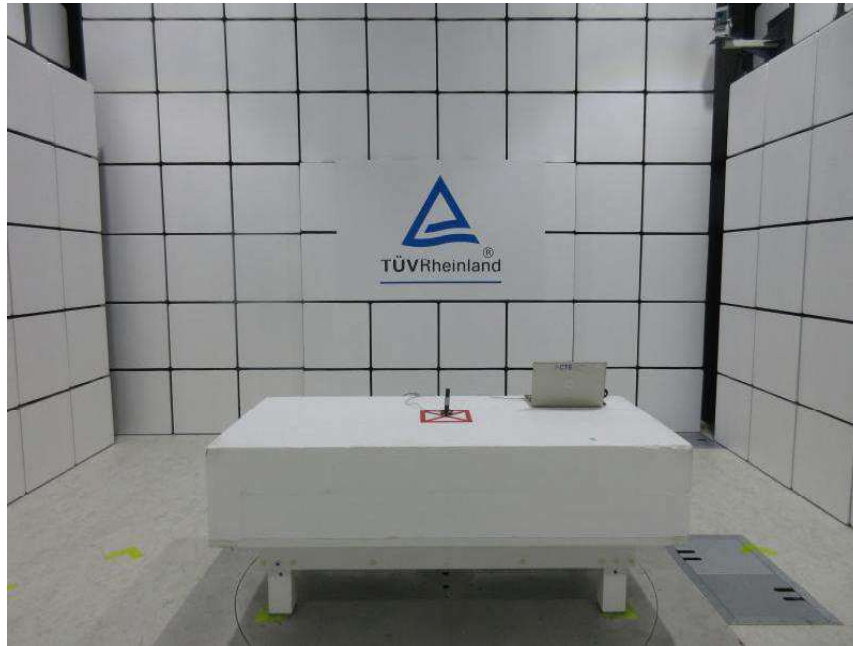
Photograph 2: Set-up for Spurious Emissions (Front View 2)
