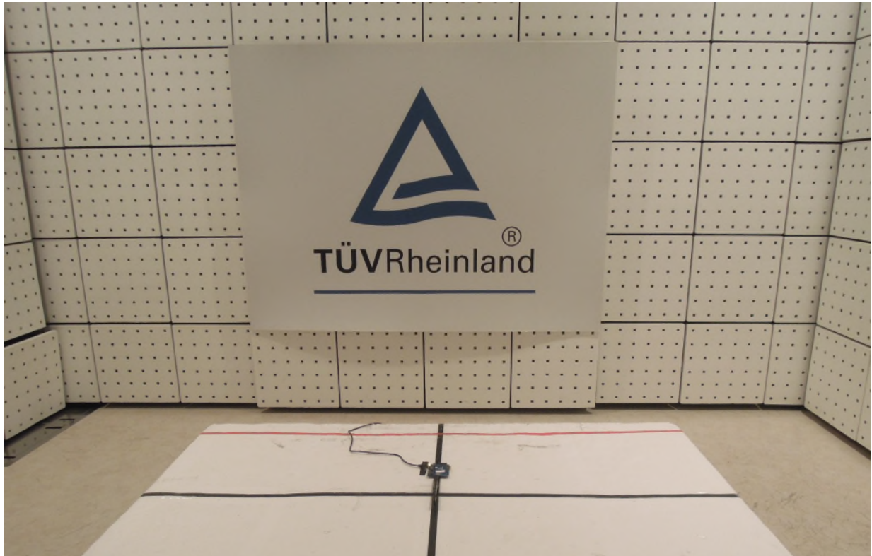
Photograph 1: Set-up for Spurious Emissions (Front View 1)
