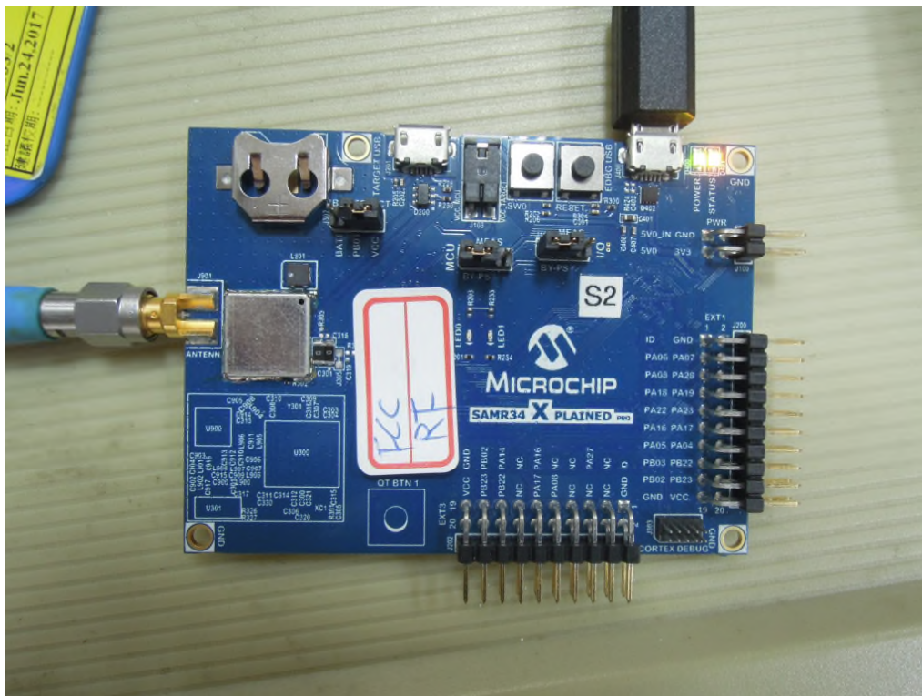
Photograph 7: Set-up for Conducted testing
