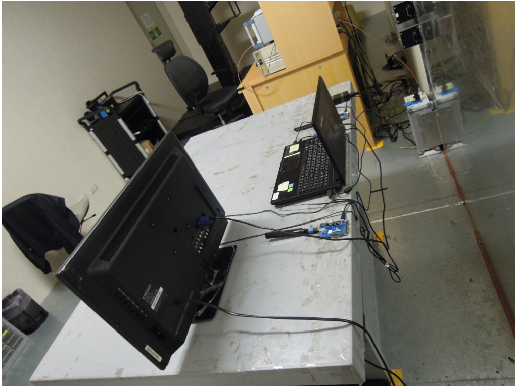
Photograph 8: Set-up for for Mains Conducted testing Back
