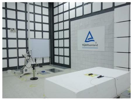
**Photograph 4: Set-up for AC Mains (Front View)**
