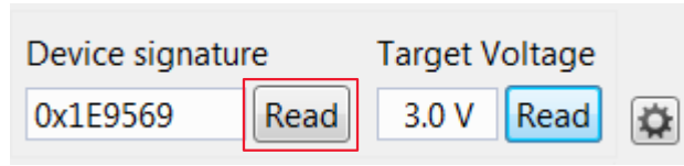
Figure 6-4. ATA5702 Signature Verification
