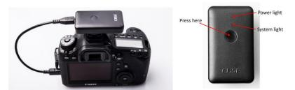
• Turn on CASE Remote Air. Press the button for more than 3 seconds to turn on CASE Remote Air. If you press the button again for more than 3 seconds, CASE Remote Air will be turned off. When the system light is blue and stable, CASE Remote Air will work functionally.
