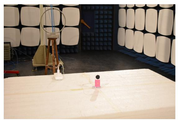
3. Radiated emission (9KHz-30MHz)
