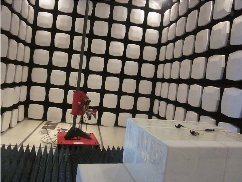
Measurement of Radiated Emission Test Set Up
