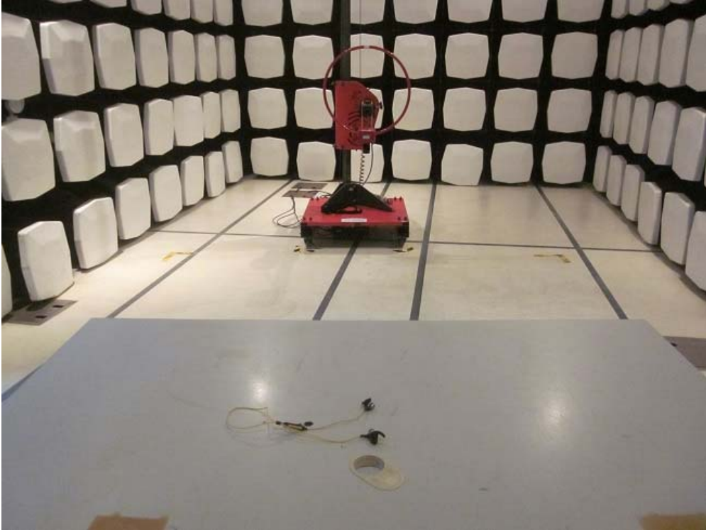
Measurement of Radiated Emission Test Set Up
