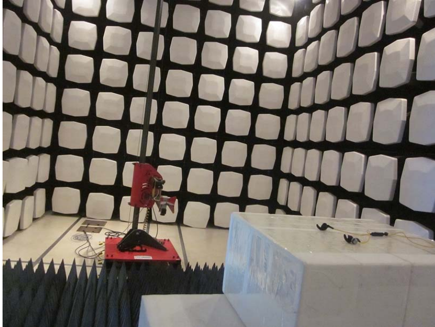
Measurement of Radiated Emission Test Set Up
