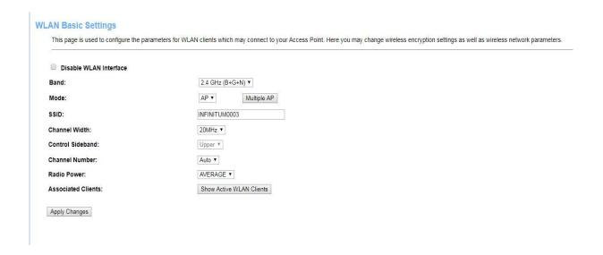
Here you may enable or disable the wireless function. You can also change the wireless parameters, such as Band, SSID, Channel Width, Control Sideband, Channel Number and Radio Power.
