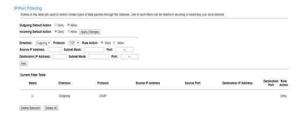
On the front of the page, you can see the default action of outgoing/incoming connection. If the IP connection doesn't match any filter rules, the router will handle the connection with the default action setting.
