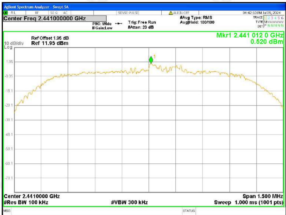
Tx. Spurious NVNT 2-DH5 2441MHz Ant1 Ref
