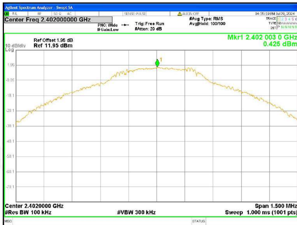
Tx. Spurious NVNT 1-DH5 2402MHz Ant1 Ref
