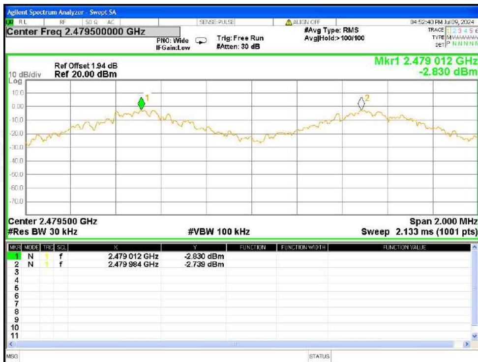
CFS NVNT 1-DH5 2480MHz Ant1
