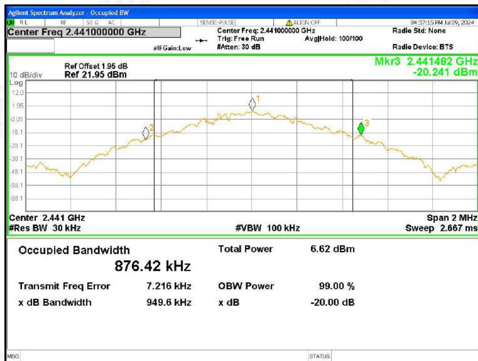
-20dB Bandwidth NVNT 1-DH5 2441MHz Ant1
