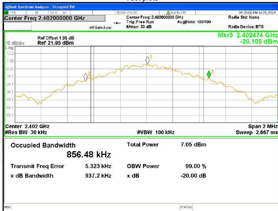
-20dB Bandwidth NVNT 1-DH5 2402MHz Ant1
