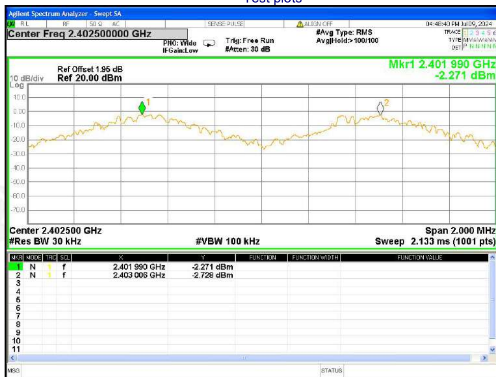
CFS NVNT 1-DH5 2402MHz Ant1
