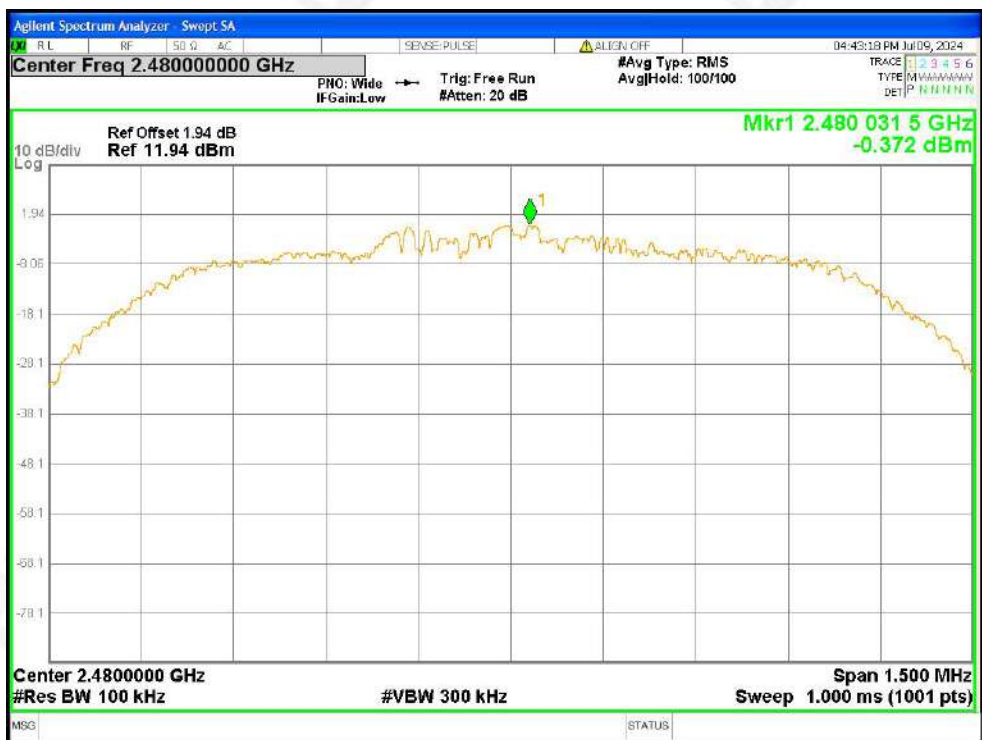
Tx. Spurious NVNT 2-DH5 2480MHz Ant1 Ref
