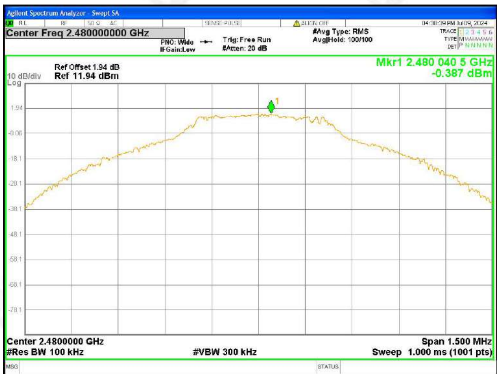
Tx. Spurious NVNT 1-DH5 2480MHz Ant1 Ref
