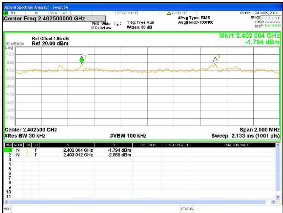
CFS NVNT 3-DH5 2402MHz Ant1
