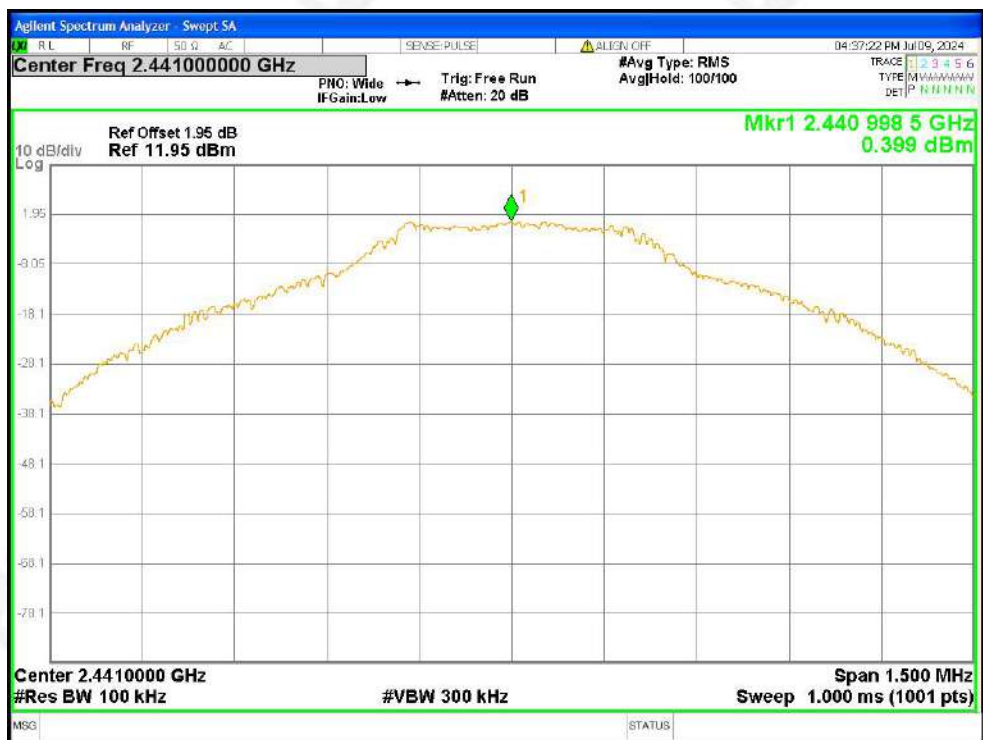
Tx. Spurious NVNT 1-DH5 2441MHz Ant1 Ref
