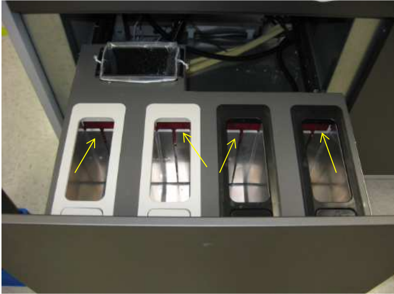
Material Distribution Module (MDM) with material bottles removed: Antenna locations are shown using arrows
