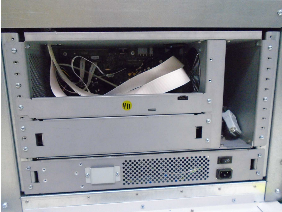
Cover removed from electronics enclosure; DMC board mounted vertically inside of ProJet® MJP 2500
