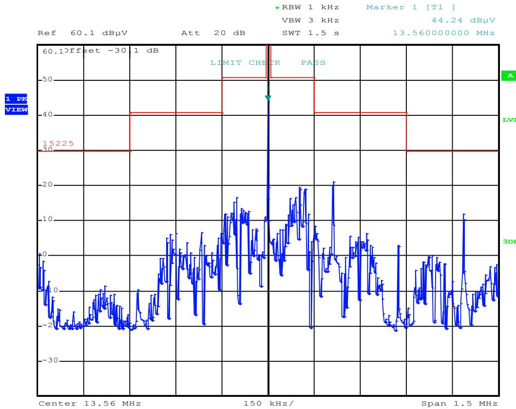
The values of the plot are extrapolated to a measurement distance of 3 m. (calculated Limit 124 dB $\mu$ V/m)
