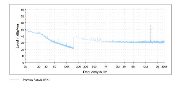
Remark: The peak at 68 kHz was caused by the measurement system and not by the equipment under test The peak at 13.56 MHz is the simultaneous transmitting RFID reader – so a wanted signal
