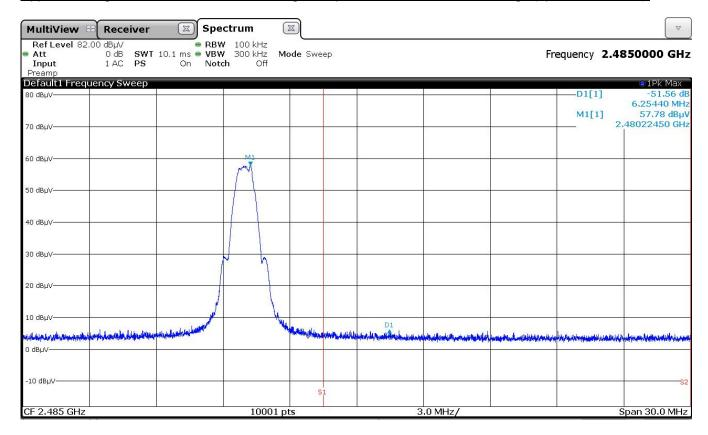
No emissions were found during the preliminary measurement; therefore no final measurement was performed.
