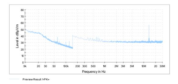
Remark: The peak at 68 kHz was caused by the measurement system and not by the equipment under test The peak at 13.56 MHz is a wanted signal of the EUT (NFC/RFID)
