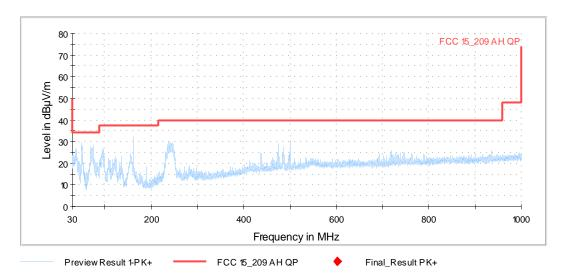
170923 1-4GHz ch00 : Spurious emissions from 1 GHz to 4 GHz (operation mode 2):
