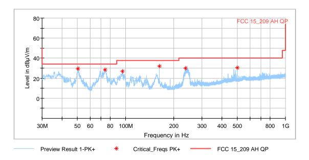
The following frequencies were found outside and inside the restricted bands found according to FCC 47 CFR Part 15 section 15.209.
