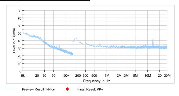
Except the fundamental of the EUT at no frequency was a value above the noise of the system therefore only a final measurement for the fundamental on the open area test site was carried out. No spurious emissions caused by the equipment under test were found.
