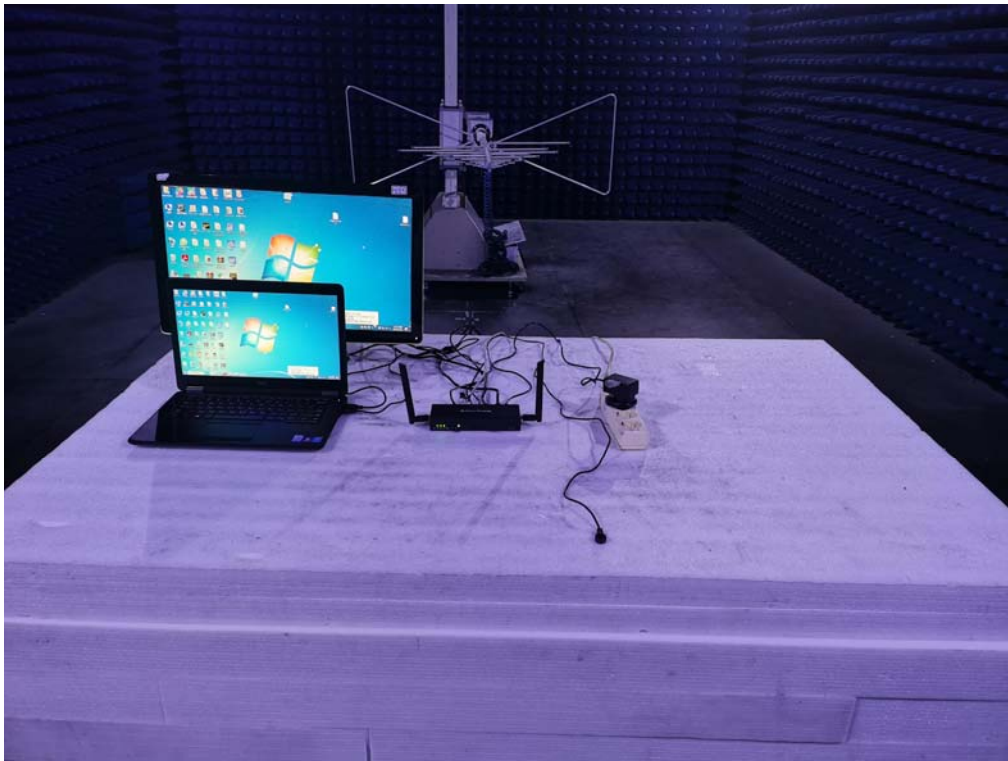
Photo of Radiated Emission Measurement (Below 1G)
