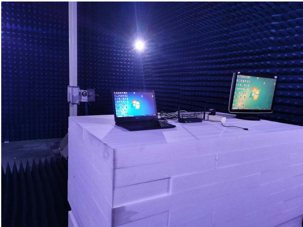
Photo of Radiated Emission Measurement (Above 1G)
