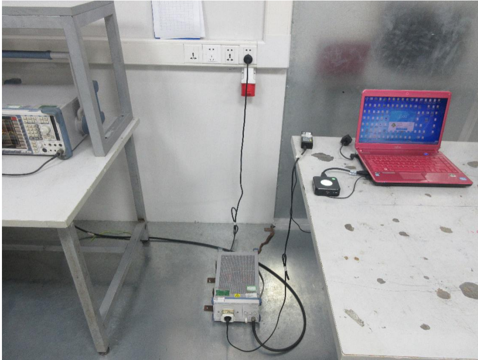
Photo of Radiation Emission Test
