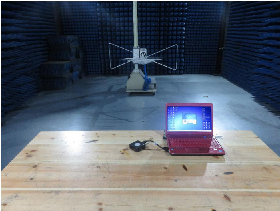
Photo of Radiation Emission Test
