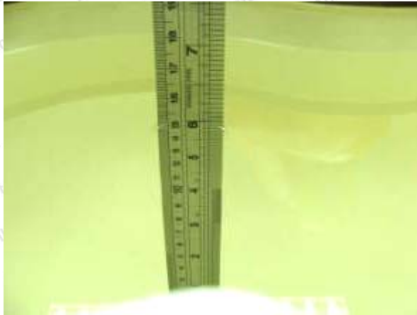
Photo of Liquid Height for Head SAR
