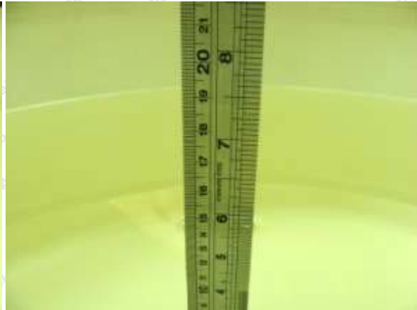
Photo of Liquid Height for Body SAR
