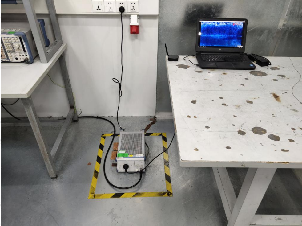
Photo of Power Line Conducted Emission Test
