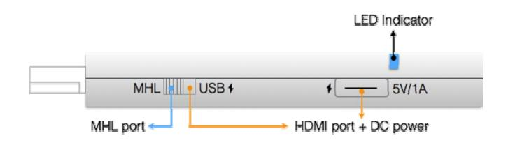
The EZCast Pro dongle is compatible with MHL interface, so there are 2 ways to connect with EZCast Pro dongle with your receiver devices like TV, Monitor or Projector. Use the switch to choose HDMI output or MHL output, please be noted your MHL device must provide 900mA power, and if you use HDMI out, you will need external 5V/1A DC power to bring up the dongle.
