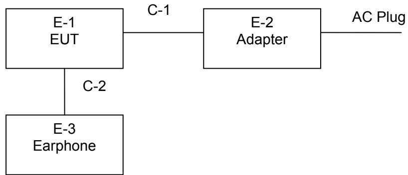
Radiated Spurious Emission Test
