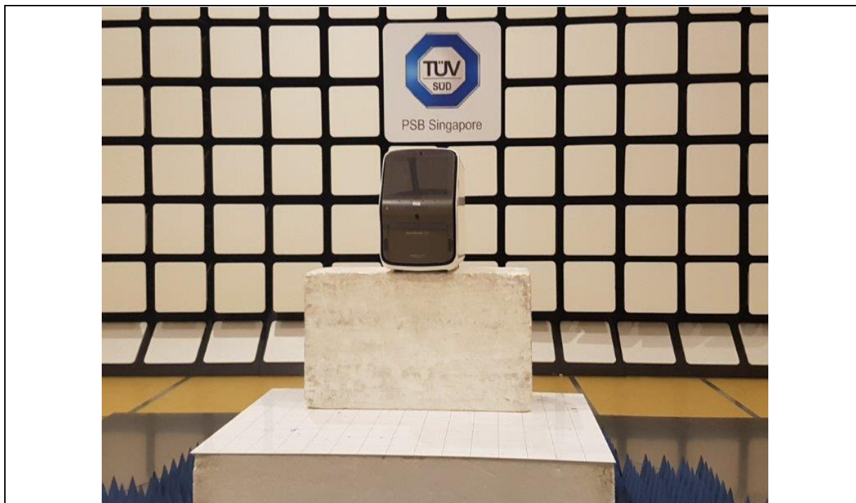
Radiated Emissions Test Setup (Front View)
