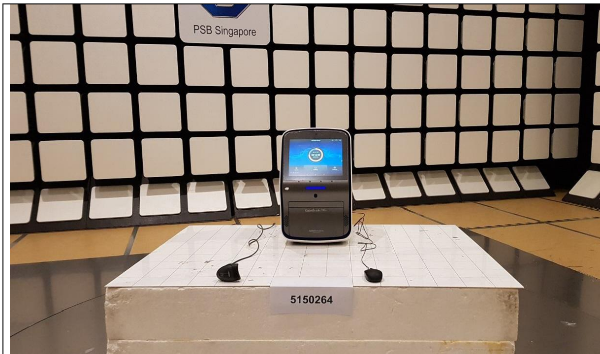
Radiated Emissions Test Setup (Front View)
