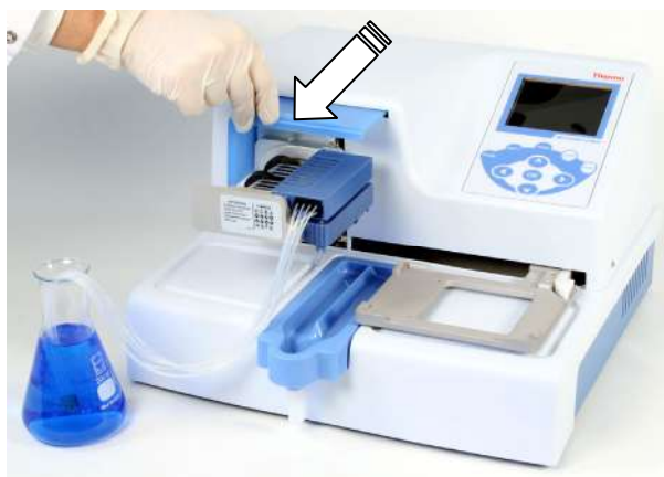
Figure 4–20. Pulling the rotor cover over the rotor
