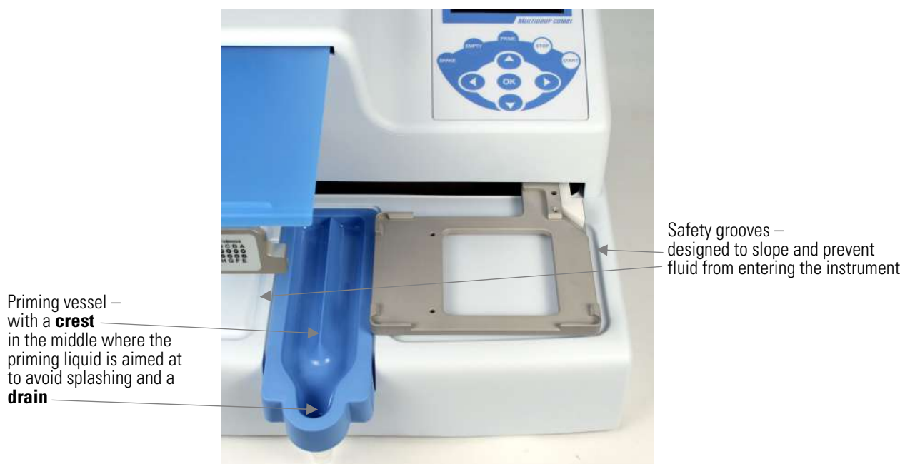
Figure 4–9. Priming vessel inserted into place
