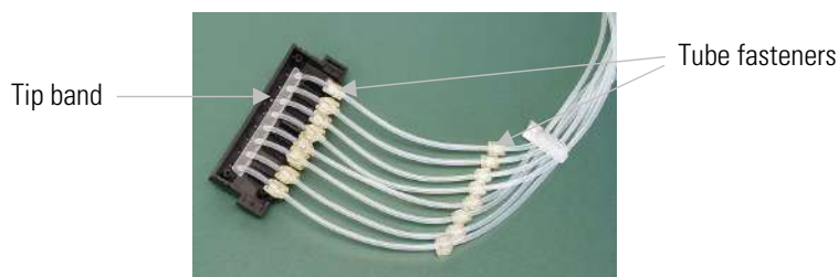
Figure 5-29. Inserting the tip manifold into the lower part of the dispensing cassette
