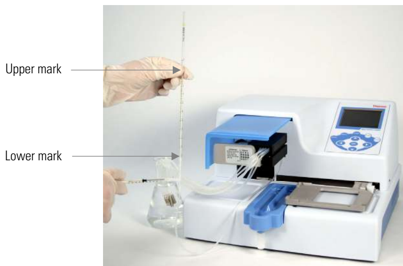
Figure 6–52. Adjusting the liquid level first to the lower mark and then to the upper mark
