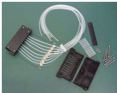
Figure 5–34. Parts belonging to the upper part of the dispensing cassette
