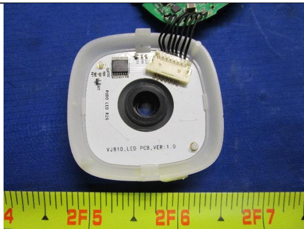
EUT – LED Board – Rear Side
