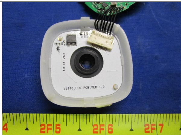
EUT - LED Board - Rear Side
