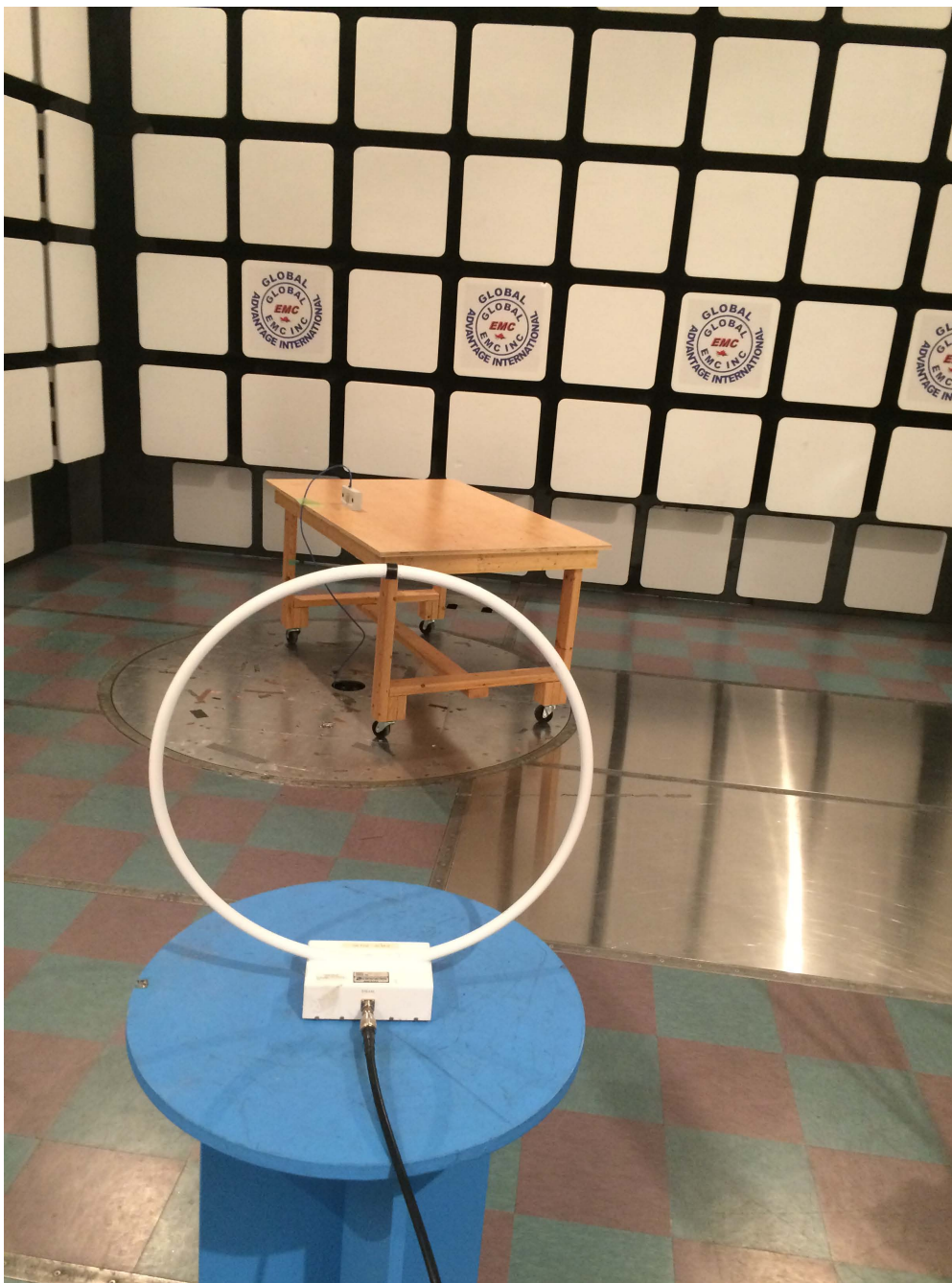
Figure 5: Radiated emission setup – photo 1
