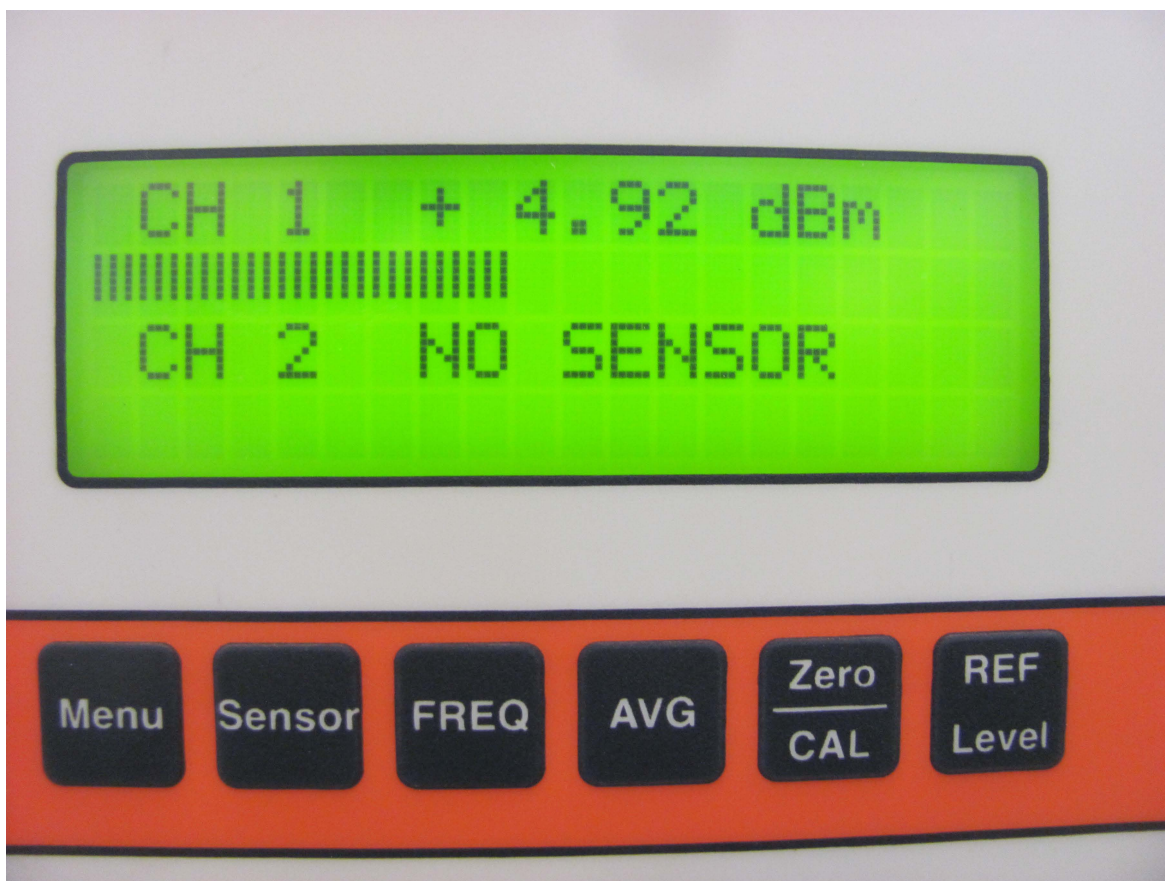
Figure 2: Power meter reading, 802.11g Channel 11– photo
