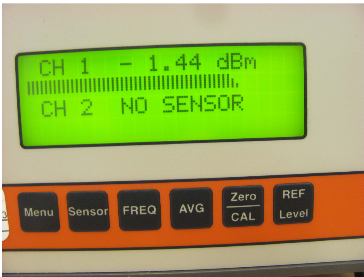
Figure 1: Power meter reading, BLE Channel 0- photo
