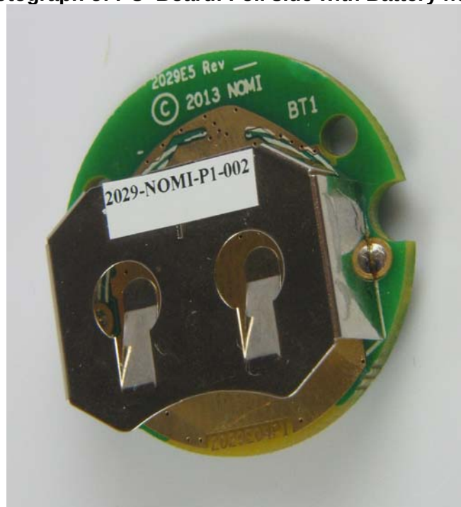
Photograph of PC Board: Foil side with Battery holder
