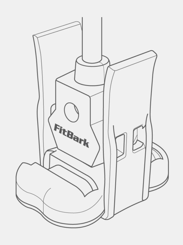
Clamp the charging cable to the FitBark GPS and plug the other end into a powered USB port on your computer. The LED will turn from flashing to solid when fully charged.
