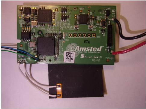
Note: The blue, black and green wires are not installed during application. They were used for test programming only.
