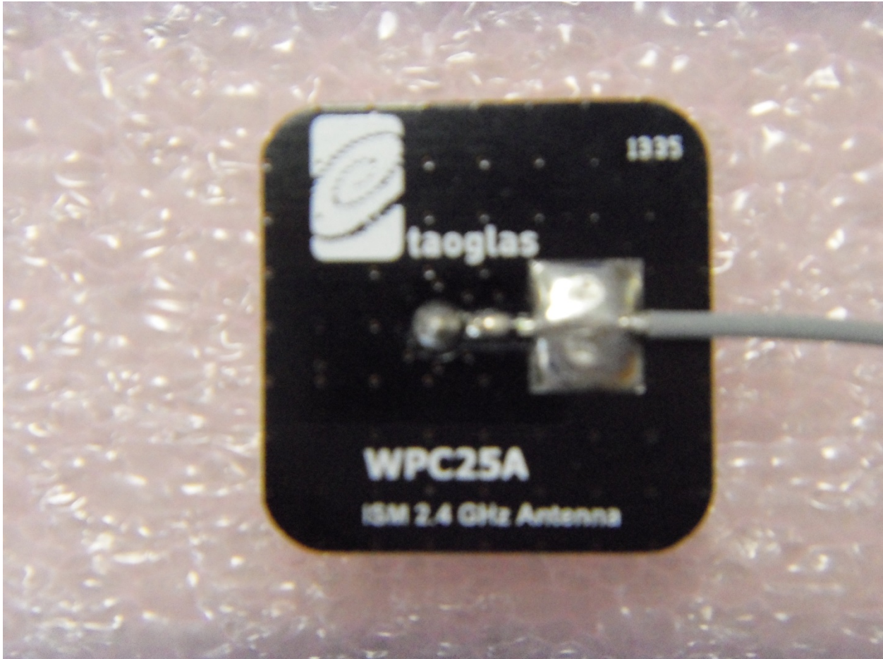
3.5 dBi Omni patch Antenna Top (Removed from Housing)
