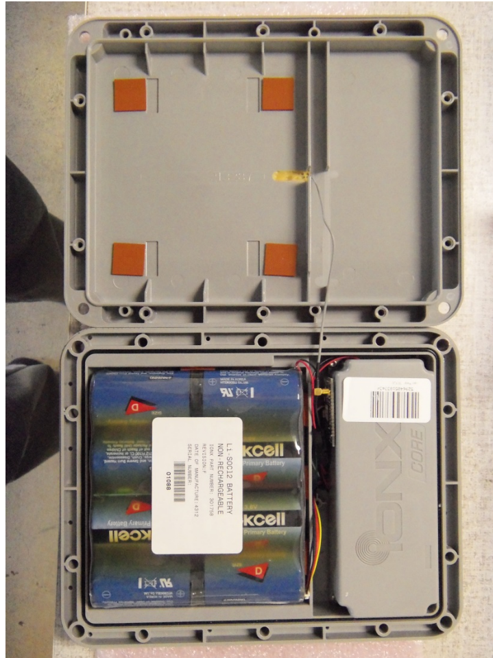
Enclosure Open, showing Batteries
