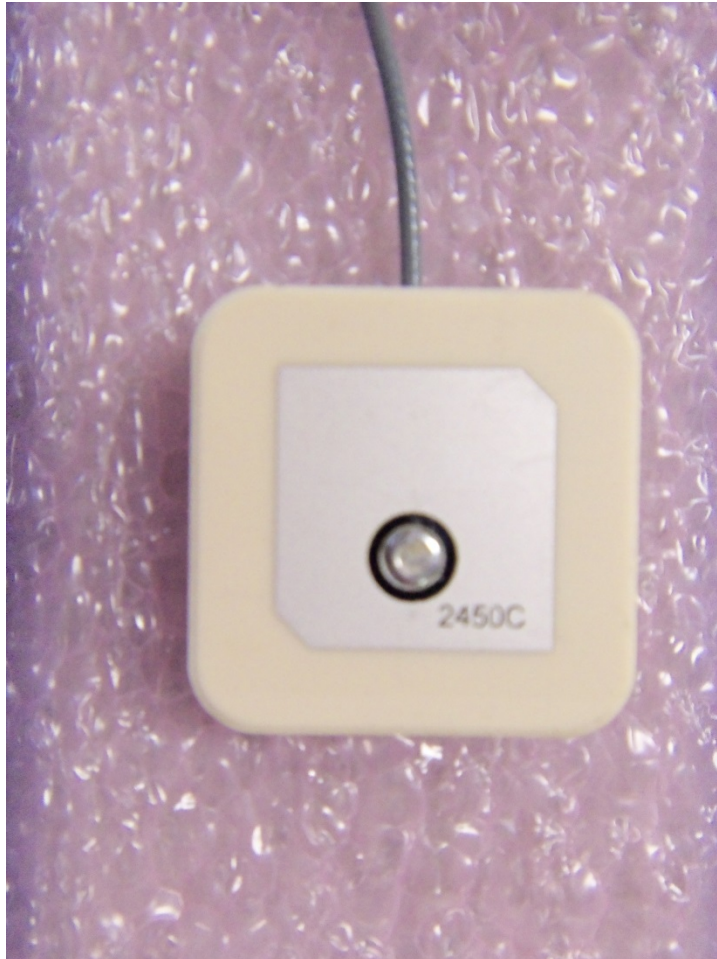
3.5 dBi omni patch Antenna Bottom (Removed from Housing)
