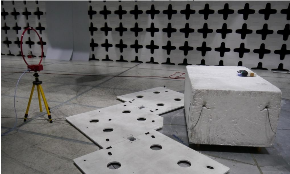
9kHz to 30MHz Setup with Co-Axial Loop Antenna
