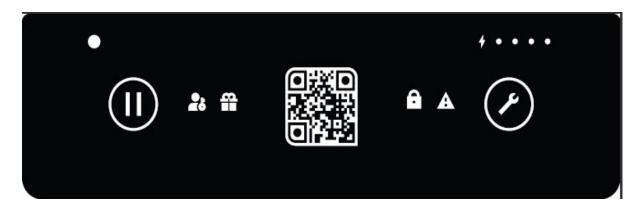
The three large circles are capacitive touch buttons intended for users to interact with. The left button puts a ride on hold, the middle button wakes up the module, and the right button reports issues with the bike. The four smaller icons are indication LEDs that indicate the following (left to right): reservation status of bike, user incentive/bounty, bike is unlocked, bike is locked.
