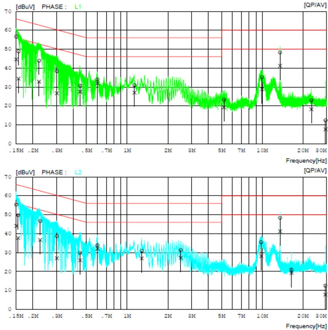
**Measurement Data****Results of Conducted Emission**
