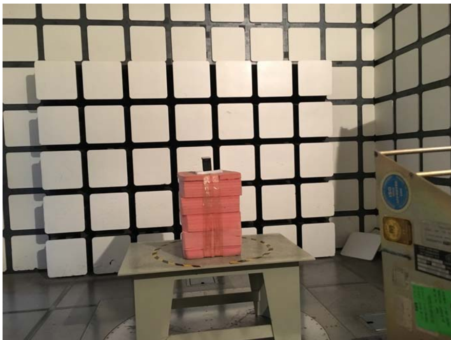
Radiated Emissions View (Above 1 GHz)
