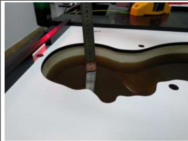
Liquid depth in the Head phantom
