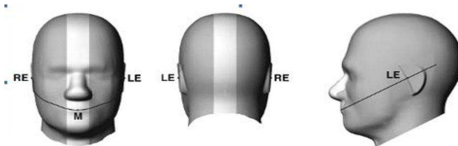
F-2. Front, back, and side views of SAM (model for the phantom shell). Full-head model is for illustration purposes only-procedures in this recommended practice are intended primarily for the phantom setup.
