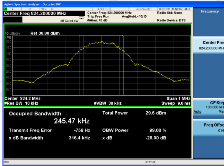
26dB&99% Occupied Bandwidth Plot on Channel 190
