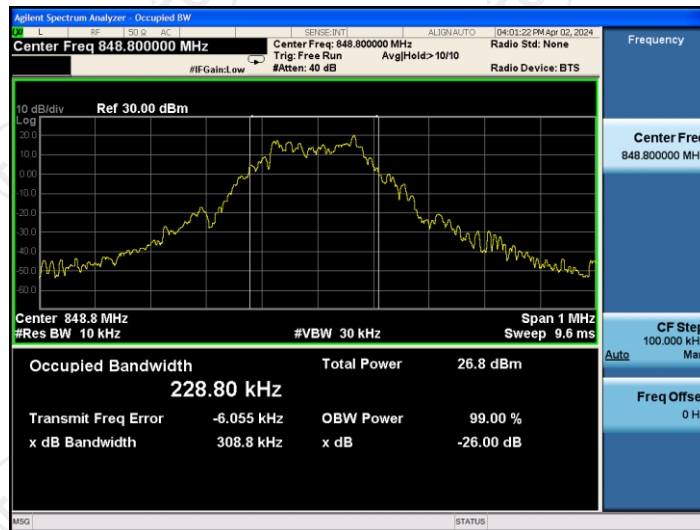
26dB&99% Occupied Bandwidth Plot on Channel 251
