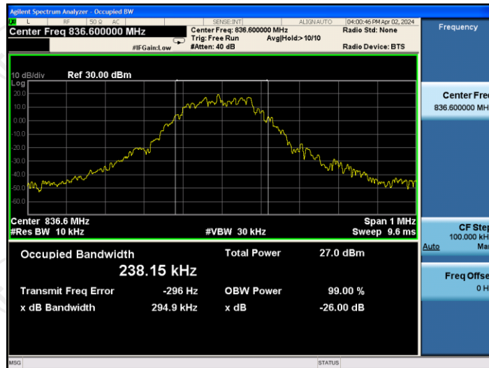
26dB&99% Occupied Bandwidth Plot on Channel 251
