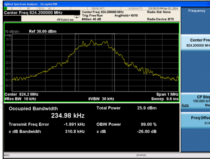
26dB&99% Occupied Bandwidth Plot on Channel 190
