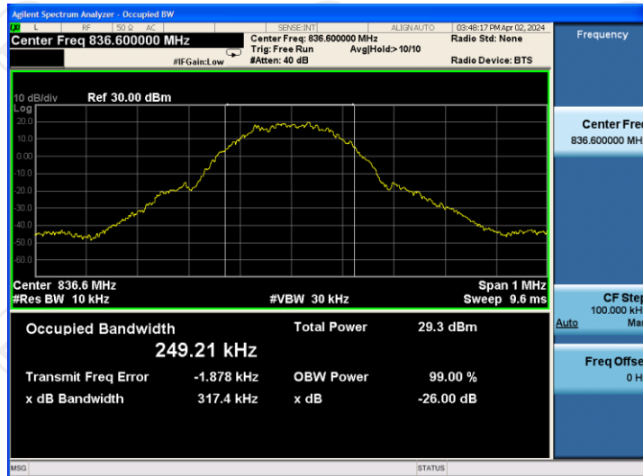
26dB&99% Occupied Bandwidth Plot on Channel 251
